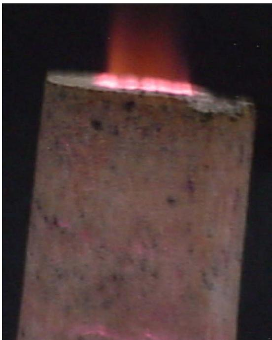
Fig. 2a. Flaming combustion.
