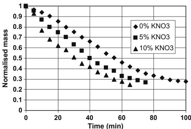
Fig. 5. Effect of oxidizer and binder on burn time.
