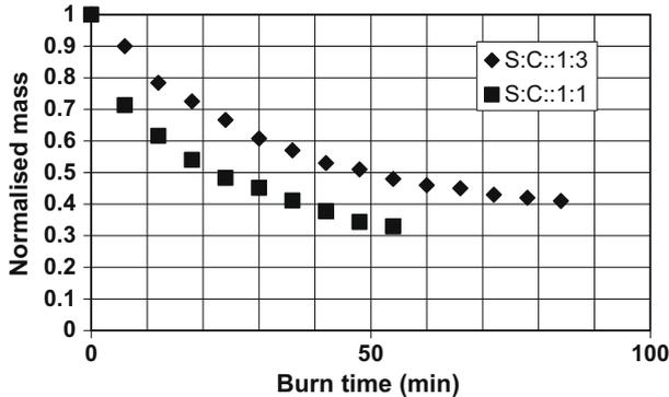
Fig. 4. Effect of charcoal on burn time (S, C represents sawdust and charcoal, respectively).
