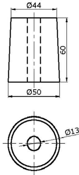
Fig. 6a. Single hole fuel block.
