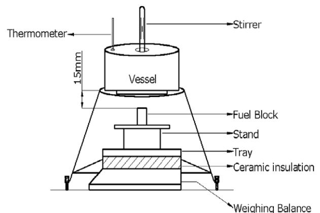
**Fig. 3.** Experimental setup for thermal efficiency test.
