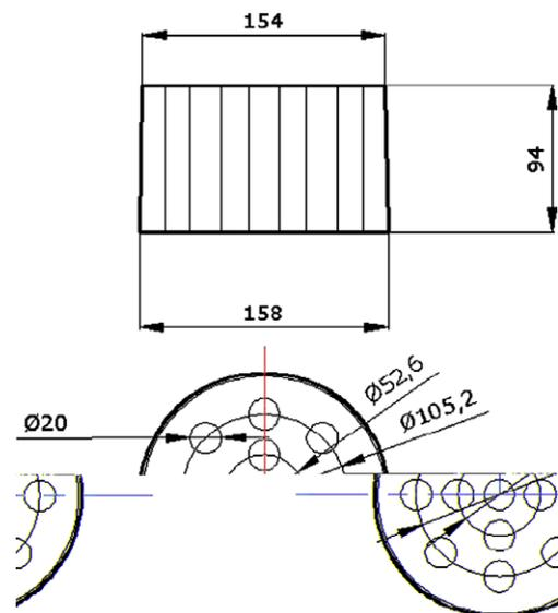
Fig. 6b. Multi-hole fuel block.
