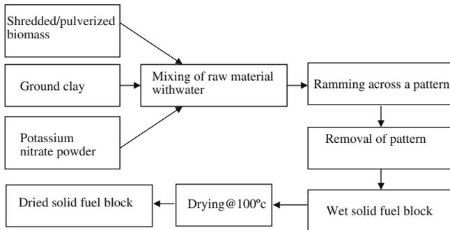
Fig. 1. Block diagram of preparation details of fuel block.
